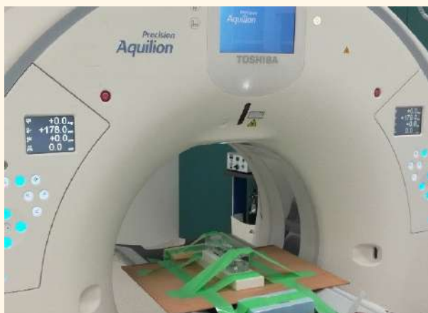
Figure 1: Handmade phantom setting in the Aquilion Precision (UHR-CT)
