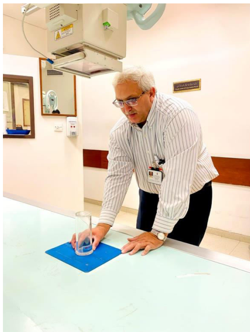
Setup to check X-ray Beam Centring and Collimation
